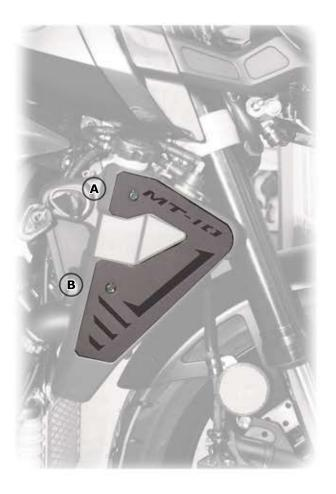
KIT X2. AIR CONTROL (RIGHT-LEFT SIDE) X4. SCREW 6X35 "ROUND HEAD" X4. THREAD
