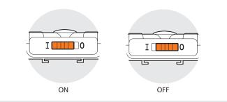
To turn on the FreeWire, slide the **Power Switch** to **I**. To turn off, slide the **Power Switch** to **O**.
